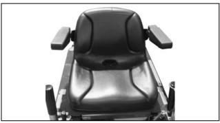
Optional Arm Rests for added comfort. Set includes left and right arm rest and mounting hardware.
